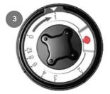
Rotate the black control knob clockwise 10 to 12 turns. This releases the galvanic element into the liquid electrolyte, thus activating the GREASOMATIC®.
