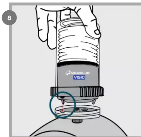
Align the pin of VISIO Module with the notch of VISIO Base.
