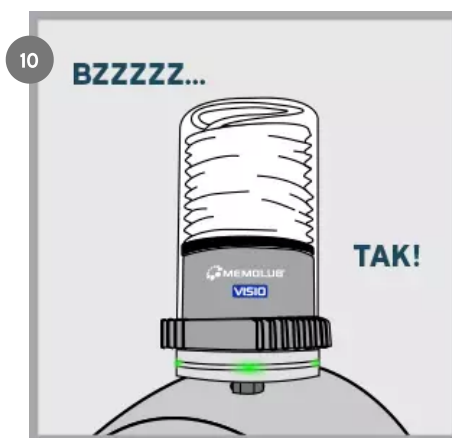
VISIO initializes, flashes each color on, and makes one expulsion. Green light confirms proper functioning.
