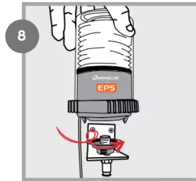
Install MEMOLUB® EPS MEMORY on Memo. Connect the cable to the 24V DC power supply.
