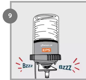
9 MEMOLUB® EPS MEMORY works immediately. NOTE: if there is no change in the settings (rings) since its last operation, the unit may not pulse immediately.
