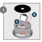
Insert new battery pack and seal. NOTE: the battery seal can be removed for 480cc cartridges.
