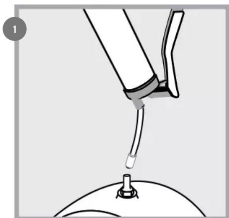
Prime lube point and remove nipple.
