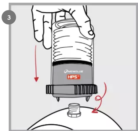
Install MEMOLUB HPS BLUE on the brass fitting.
