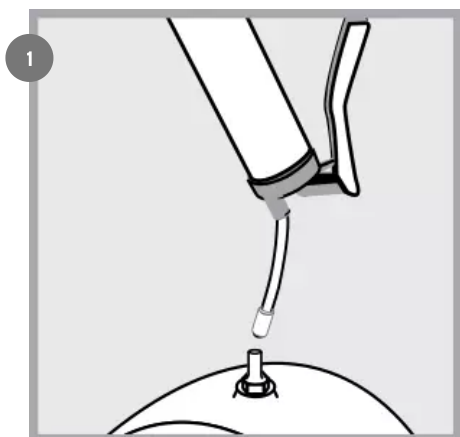
Prime lube point and remove nipple.
