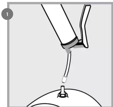
Prime lube point and remove nipple
