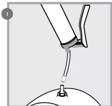
Prime lube point and remove nipple
