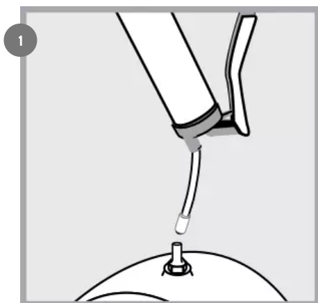
Prime lube point and remove nipple.
