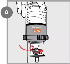
8 Install MEMOLUB® EPS MEMORY on Memo. Connect the cable to the 24V DC power supply.
