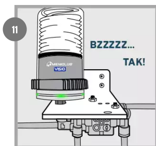
VISIO initializes, flashes each color on, and makes one expulsion. Green lights confirm normal operation.
