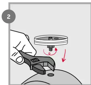
Install VISIO Base using a strong threadlocker (BSP 1/4).
